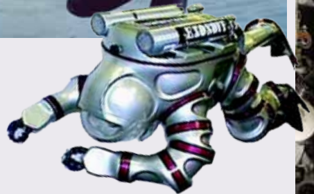
The Exosuit Swimmable ADS is self-contained, autonomous and free-swimming. It has basic pincer manipulators or a four-fingered prehensor "hand."
